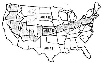
AREA I- INTERLAYERS ARE RECOMMENDED WITH MINIMUM OVERLAY THICKNESS OF 2 IN.
