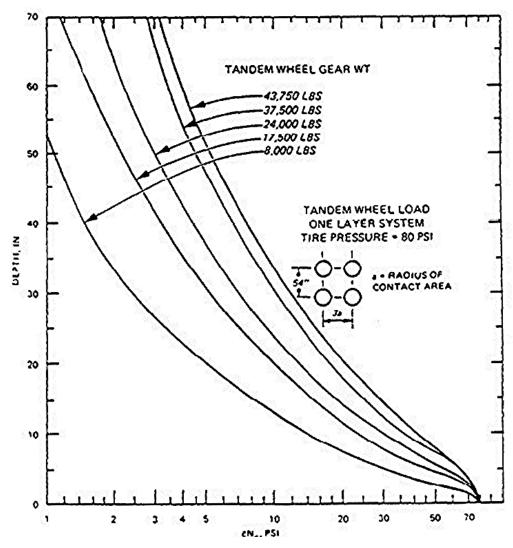
Thickness Design Curve for Tandem- Wheel Load on Gravel-Surfaced Roads
